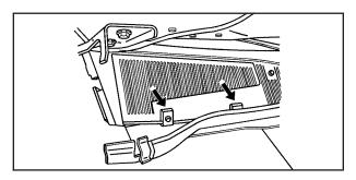
Push the two tabs on the access panel door towards the windshield.
